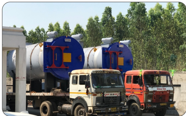
SML Ltd. - Surat, Gujarat Thermic Fluid Heater:- Capacity- 25,00,000 Kcal/hr x 2, Fuel- Furnace Oil cum Natural Gas
